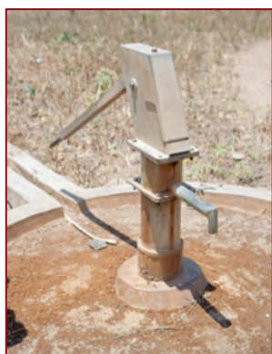
Reliability and availability of spare parts. India Mark II hand pumps are robust with available spare parts in PNG. (source: Wikipedia )
