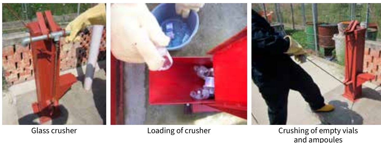
Fig. 17 Use of Médecins Sans Frontières glass crusher on empty vials and ampoules
