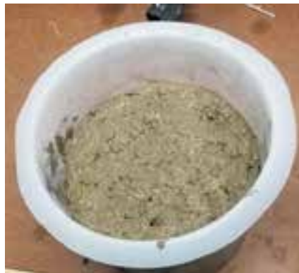
Mixing of cement and pharmaceutical waste
