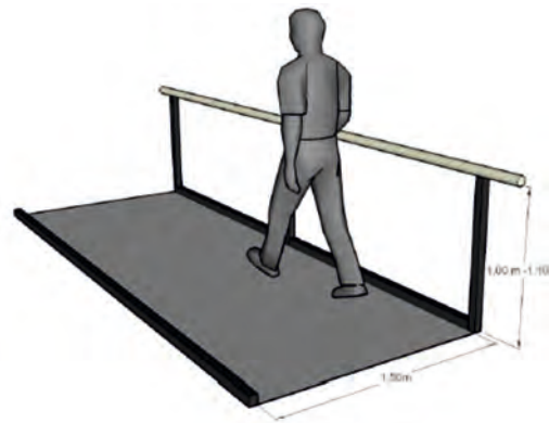
Typical inclined ramp. Source: Handicap International
